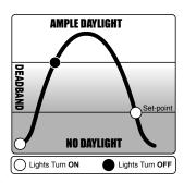
the set-point. There is also a 20 minute delay before the sensor switches the lights off to prevent the system from cycling on a cloudy day; and a 45 second delay before switching from off to on. ".
